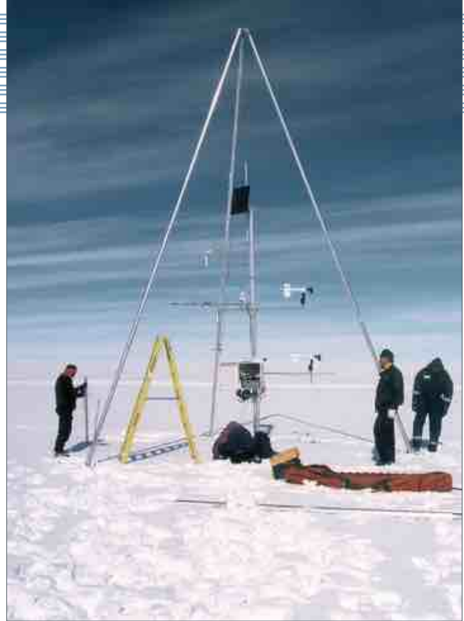
A weather station begins to lean with recent snowmelt. Researchers rode snow-mobiles to steam-drill a new 6-meter (20-foot) hole and secure the station. Credit: John Maurer
